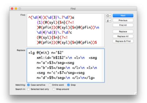
The TEITagger driver file also accepts commands to insert header and footer files so that one can add the opening XML file tags, open and close body and text tags, open and close TEI tags, and a teiHeader. Finally, TEITagger will pretty print the file if it is a valid XML file.
